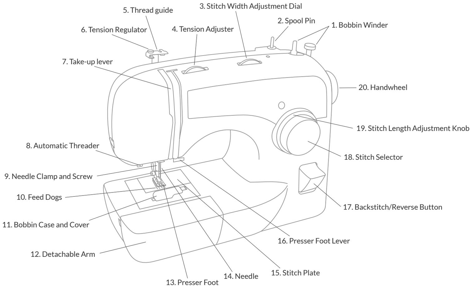
**1. Bobbin Winder** - Used to wind thread onto a bobbin cases. Locks into place to engage the bobbin winding motor and not the main sewing motor.
